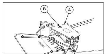
Figure 19. Belt Cover A. Belt Cover Plate B. Belt Cover Latch
